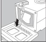
4. Very carefully slide out the right polythene bag, removing it towards the left and then upwards. Remove the bottom cover placed into the drum of your appliance, lay it's hook as the arrow 'A' indicates and push the top of the cover to seal it closed
